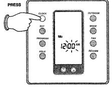
Step 3: Press the CLOCK button again and "12:" (hours) and "AM" or "PM" will flash. Use the DECREASE or INCREASE button to change the flashing symbol to the current hour making sure the hour has the proper AM or PM designation.
